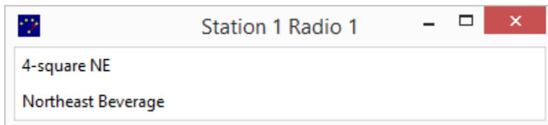
Since this display only shows the selected antenna it cannot be used to choose a different antenna.
