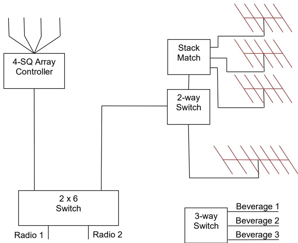
The beverages show antennas which are receive-only. It is not necessary to press the RX button before selecting one.
