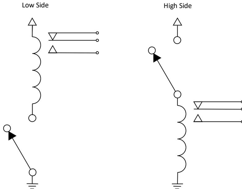
The relays are connected to pluggable block (Phoenix) connectors. Each connector supports eight relays. The connectors also have two pins which are connected to either +V or ground, determined at construction time.
