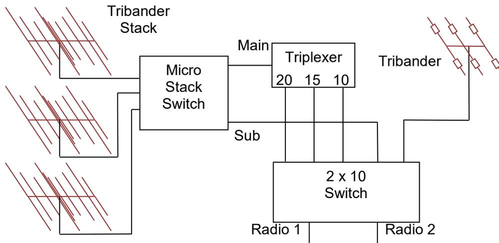
The triplexer allows both stations to use the same antennas.
