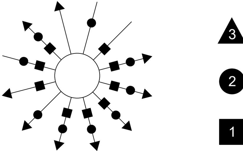
This scheme shows *exclusive antennas*. Each position selects an exclusive combination of antennas. (There are several positions which select all antennas because the switch they used had 12 positions).
