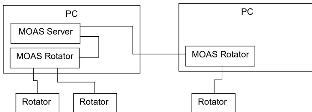
There is no practical limit on the number of computers running MOAS Rotator or on how many rotators are connected to each computer.
